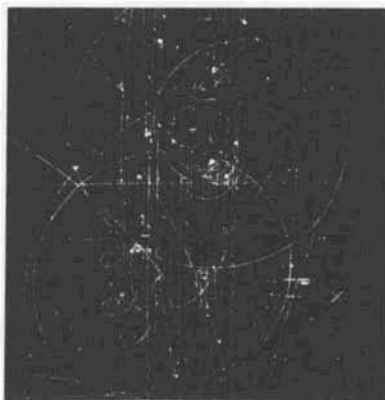
FIG. 11-7. A liquid-hydrogen bubble-chamber photograph of a \pi^+ decaying into a \mu^+ , which decays into an e^+ . (Courtesy Brookhaven National Laboratory.)
