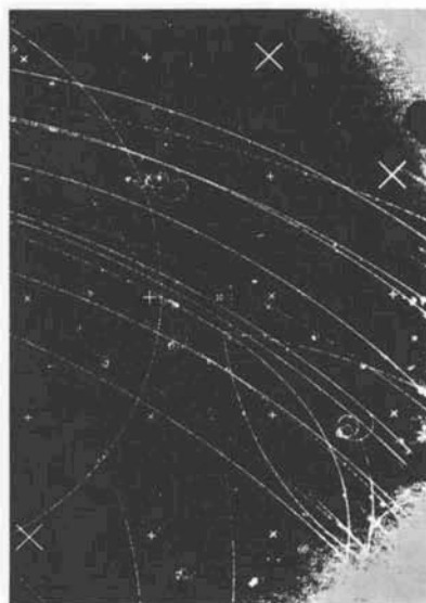
FIG. 11-8. (a) A bubble-chamber photograph of a K^- meson decaying into two pions. (b) A bubble-chamber photograph of a K^- meson decaying into three pions. (Courtesy Yale University and Brookhaven National Laboratory.)
