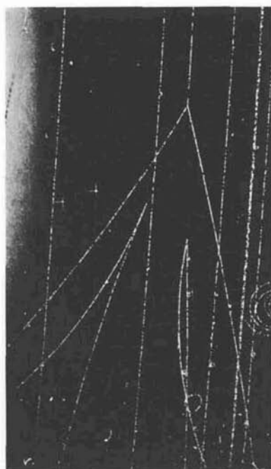
FIG. 11-10. A bubble-chamber photograph of a 2.85-GeV proton colliding with a proton and creating a K^0 and a \Lambda^0 . The K^0 decays to two pions. (Courtesy Brookhaven National Laboratory.)
